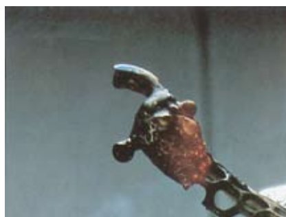
63 Heat the solder joint from the bottom to the top. When the solder reaches flow temperature, it shoots into the soldering gap.
