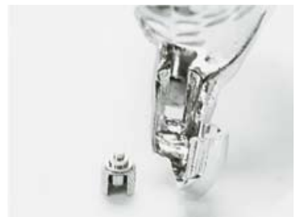
28 Unscrew the retention screw No. 387 and remove the threaded cap No. 384 from the DUOLOCK patrx.
