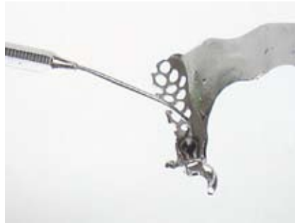
57 Coat the threads of the threaded cap with antiflux, e.g. Context (Degudent).
