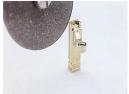
91 The matrices are shortened to the height of the patrices using a suitable rotary grinding instrument.
