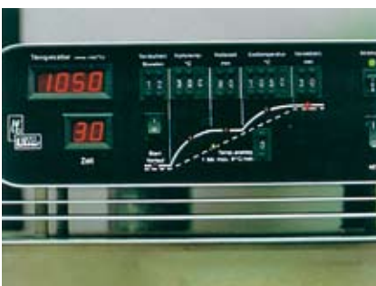
47 To avoid overoxidation of the positioning screw, the mould should not be held at the final temperature (950-1050°C) for longer than 30 minutes.
