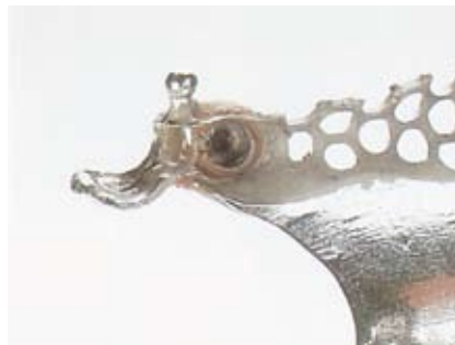
60 Ensure that the flux has flowed completely round the threaded cap.
