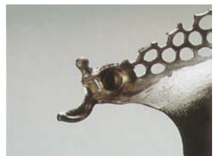
64 Check that the solder has flowed completely round the threaded cap. If a solder model was used, remove investment residue from the threaded cap after soldering with an ultrasonic cleaner or using the manual cutter No. 383. Prepare the solder joint and then insert the patrix in the threaded cap.
