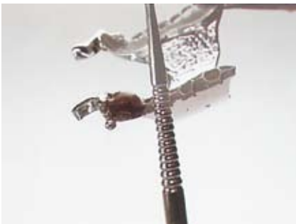
59 Vibrate the CrCo framework with an instrument to ensure the flux flows into the solder gap.
