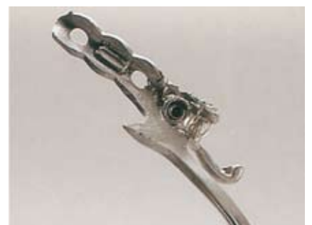
49 Clean any residual investment still sticking to the surface of the threaded cap with the manual cutter No. 383. Use oil as a lubricant.
