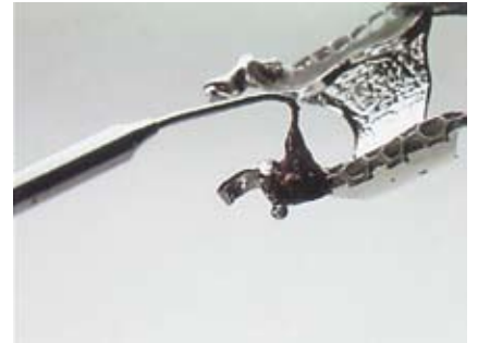
58 Apply flux, e.g. Oxynon (Degudent), to the threaded cap and CrCo framework.
