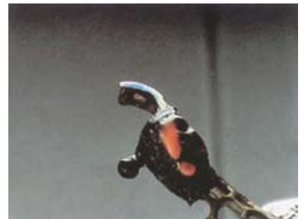
61 Degas the flux with the flame before soldering.
