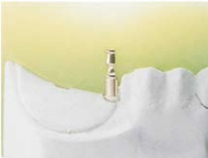
41 After the model has set, the threaded cap is fixed rigidly on the model.
