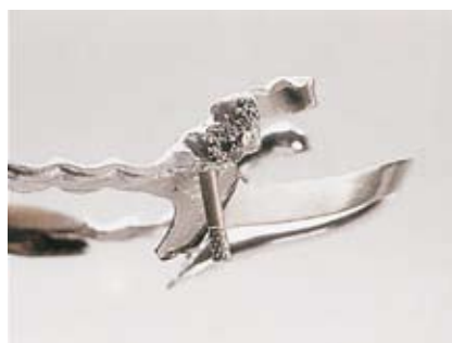
48 Cast the CrCo framework in the usual way and sandblast it after devesting. The inside of the threaded cap should only be sandblasted briefly. We recommend sandblasting the threaded cap with microbeads to prevent it being damaged. Remove the positioning screw from the threaded cap.
