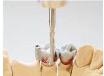
67 Mill a stress-breaker arm with interlock.
